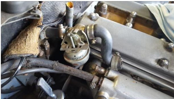
This heater valve is not original, but it works, so I'll worry about that in future years!
