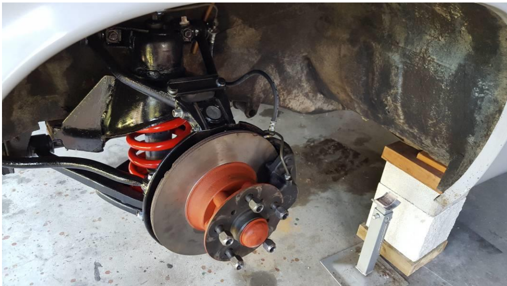
Just waiting for the road wheel. Note the chips on the brake rotor I talked about in a previous article.
