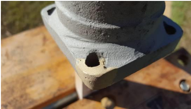
This weld repair will be invisible when the manifold is painted - with high-temp paint of course!
