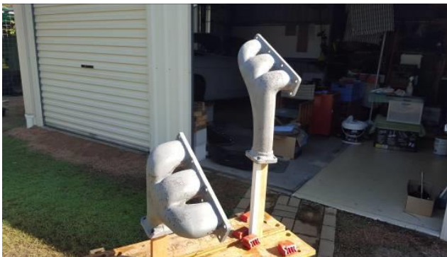
The manifolds, freshly sand-blasted and waiting for a protective coat of paint.
