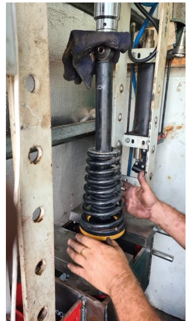
On the right - Chris, the coil-over shock unit, hydraulic press, and a safe pair of hands ...
