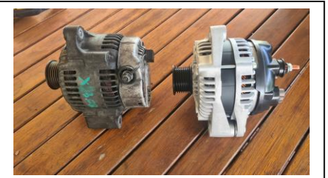
The old alternator was obviously not original. It's marked X308
